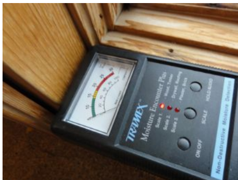
No moisture evident at stained area of window framing.
